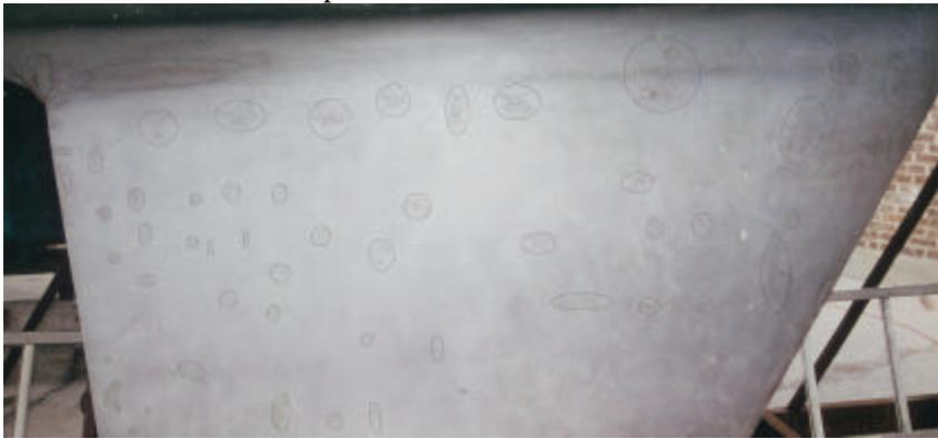
The patterns display the dendritic structure typical of the branching nature of sparks, as shown in the magnified photo below, and indicate how important sparks were during the grounding process in this strike.
