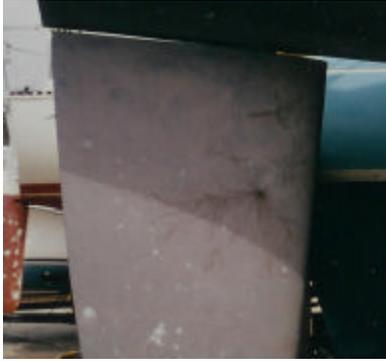
However, there was also evidence that many other sparks formed from keel ballast, bonded through-hulls, propeller shaft, and a transducer. The arcing patterns on the lead keel were much smaller in size, typically a few inches, and more closely spaced as shown in the photo below. The outer limit of each arc pattern has been marked with an ellipse.
